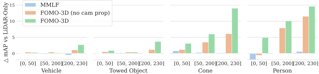
Figure 5: [Highway] Per-class mAP gains over the base LiDAR-only detector, for distance buckets [0, 50], [50, 200] and [200, 230] meters relative to the SDV. FOMO-3D (no cam prop) corresponds to M_2 in Table 4.
