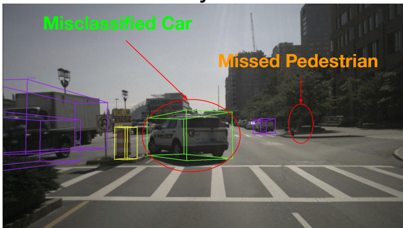
Figure 8: [nuScenes] Qualitative example #2. In this example, OWL correctly detects and classifies an adult and an emergency vehicle. The LiDAR-only model misses the adult (because it is small and sparsely observed by LiDAR) and misclassifies the emergency vehicle as car due to lack of semantics. FOMO-3D is able to successfully detect the adult thanks to OWL, but fails to retain the original OWL emergency vehicle classification.
